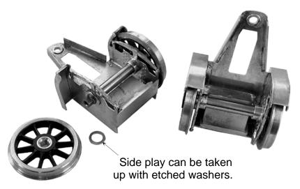
Finally to complete the bogie fold down the rear side supports and solder the nickel silver washers 70 either side of the pivot hole then add the cast weight. Repeat for the other bogie.
