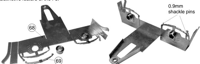
Take a bogie etch 68, they are both identical, and form the detail on reverse. Add nickel silver spring overlays 69 to the outside and shackle pin detail from 0.9 rod. Add the axle bearings. Fold up the guards at the first fold then fold down the front and fold round the sides. Tack solder in position. Fit the wheels and check for free running, reaming the bearings if necessary. Side play can be taken up with etched washers.
