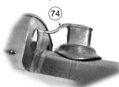
If using the early encased safety valve bonnet one will need the etched levers 74 soldered together.
